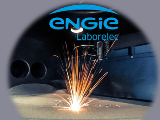
Laser Powder Bed Fusion
