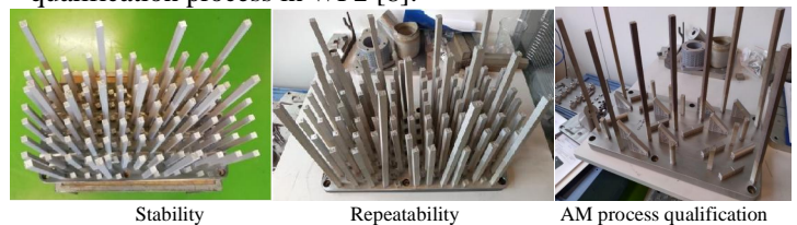
FIGURE 5: QUALIFICATION STEPS REALISATION
