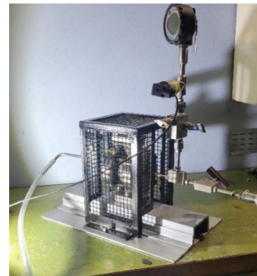
FIGURE 10: BURST TEST BENCH WITH SAFETY CAGE
